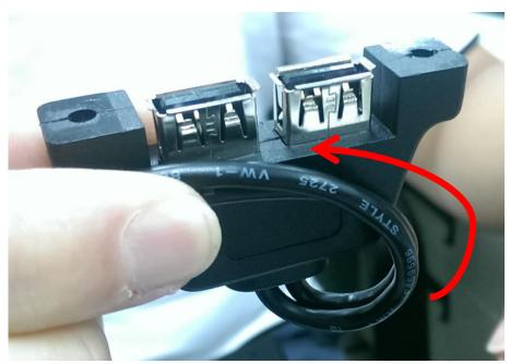
Step 2. Put the USB2.0 front panel into the chassis as following picture.
