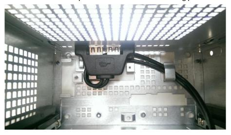
Step 3. Screw the USB2.0 front panel on the chassis as following pictures.
