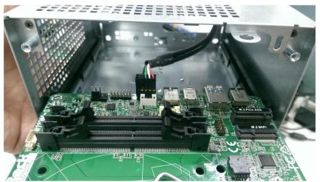
Step 5. Insert the motherboard into the chassis.
