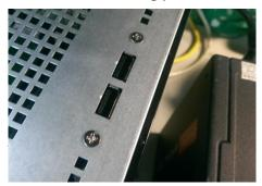
Step 4. Install the USB2.0 connector to USB2.0 header.
